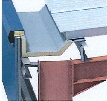
Connection to Main frame – Boundary Wall Gutter
