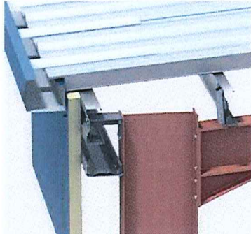
Connection to Main frame – External Gutter
